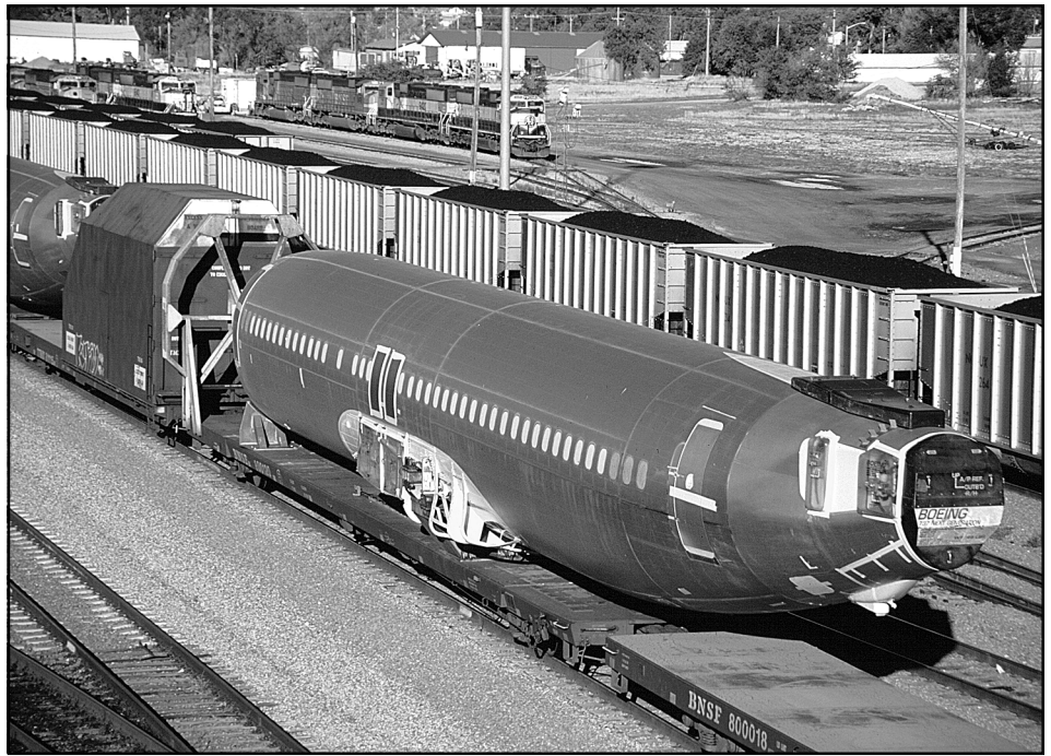
Boeing moves 737-800 fuselages from Kansas to Renton, WA, via BNSF through Alliance, NE. The Kansas City, MO, to Portland, OR, train V KCMPTL8 03A, had two fuselages on it. — October 4, 2003 photo © Chip.
